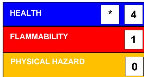
HMIS® ratings are based on a 0-4 rating scale, with 0 representing minimal hazards or risks, and 4 representing significant hazards or risks. The "\*" represents a chronic hazard, while the "/" represents the absence of a chronic hazard.
